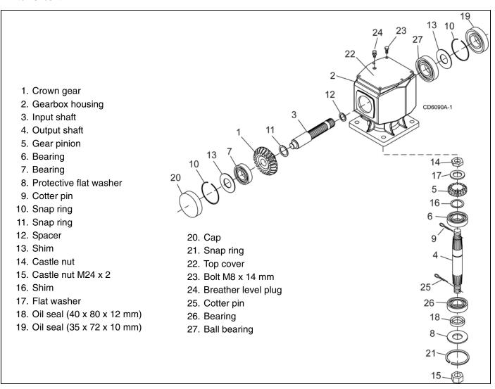
Figure 18. Gearbox Assembly
